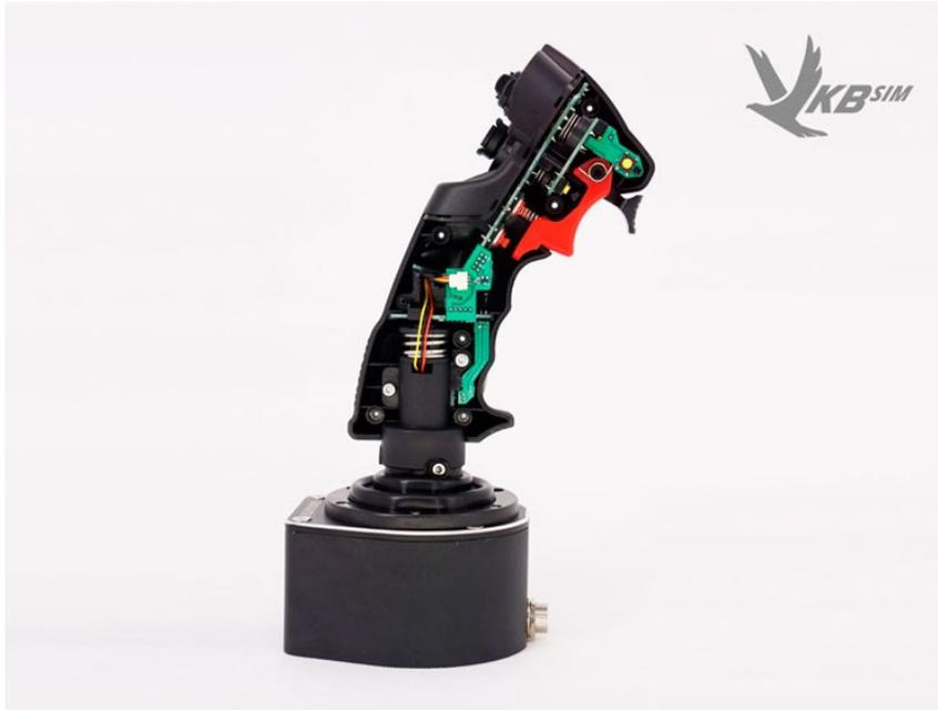
Similar to VKB's Modern Combat Grip (MCG), the Kosmosima takes its construction modularity to a new level, as there's only one 3-wire cable inside, which runs from the grip to the base connector (see image on the left).
